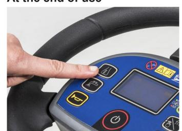
12. Machines with EcoFlex: Always turn off the detergent 2 minutes before finishing by pressing the detergent button to rinse out detergent from the system and brush before handling and cleaning.
