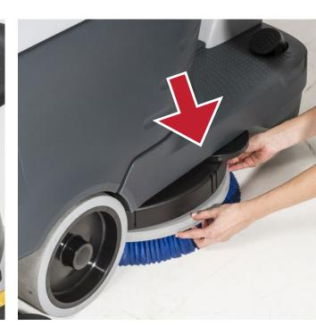
**2.** Check if the brush is correctly installed and not worn out or if there are external materials preventing brush rotation.
