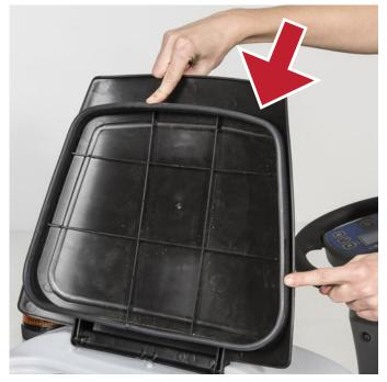
**4.** Check to see if the lid gasket is in good and working condition and sealing when the lid is closed.
