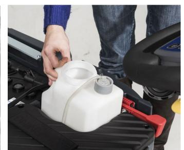
3. Fill the EcoFlex<sup>™</sup> tank with a detergent suitable for cleaning machines (highly concentrated and low foaming detergent).
