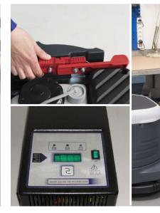
19. Charge the batteries: Connect the battery charger cord to the electrical outlet.
