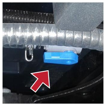
2. Check if the solution valve is open. 3. Check to see if the solution filter
