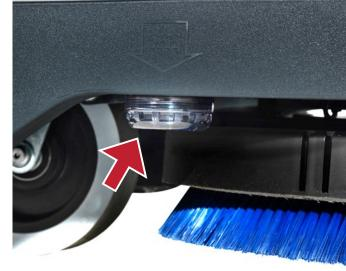
15. Clean the filter:A) Close the solution valve under the machine.B) Remove the transparent cover and the gasket, then remove and clean the filter inside.C) Reassemble the filter.
