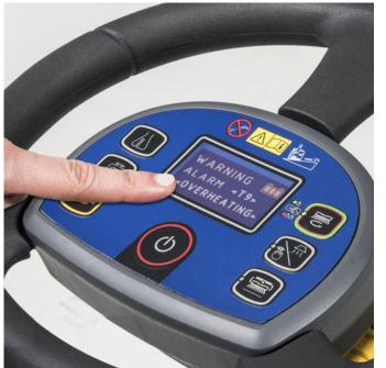
**3.** Check that floor inclination is not exceeding specifications.
