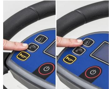
9. To change the solution flow level push the solution button and change the flow level according to the cleaning performance and application.
