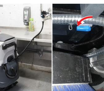
2. Fill the tank with clean water. The water temperature must not exceed 40° C.
