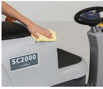
18. Clean the machine using a damp cloth and when needed use a neutral cleaning product.
