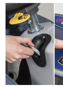
6. Insert the operator key, then start the machine by pressing the One-Touch button.
