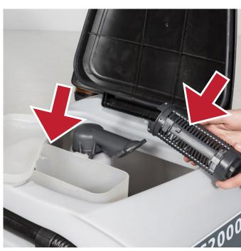
**2.** Open the recovery tank and check **3.** that the debris tray and float are clean and working.
