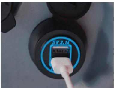
**Operator safety is paramount. A USB connection at the steering column allows the operator to keep their mobile device charged in the event of unforeseen circumstances or an emergency.**
